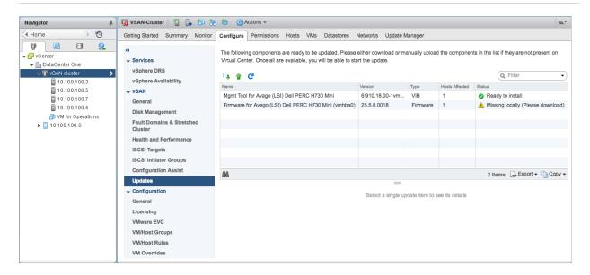
Configuration Assist verifies that your storage controllers use the latest driver and firmware version according to the *VMware Compatibility Guide*. If controller drivers or firmware do not meet the requirements, use the Updates page to perform driver and firmware updates.
