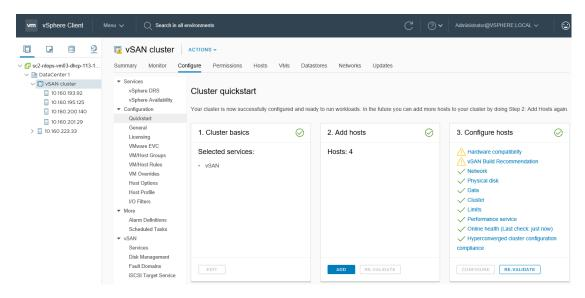
Quickstart uses the vSAN health service to validate the configuration and help you correct configuration issues. Each Quickstart card displays a configuration checklist. You can click a green message, yellow warning, or red failure to display details.
